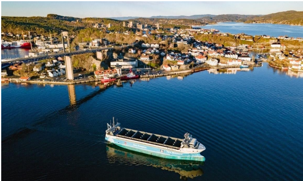
Figure 2 Yara Birkeland, the world's first autonomous and zero-emission container vessel
