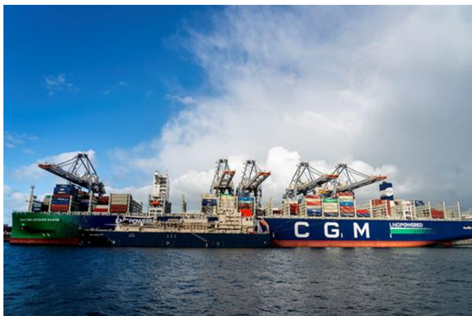
Figure 1 “Gas Agility”, the world’s largest LNG-bunkering vessel, LNG bunkering to the world’s largest LNG-fueled container ship
