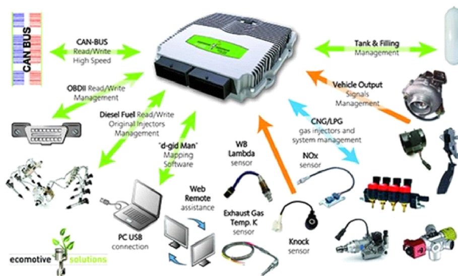
Figure 5 - BI-FUEL LNG / DIESEL, Diesel cycle engine by means of gas and diesel (compression ignition)
