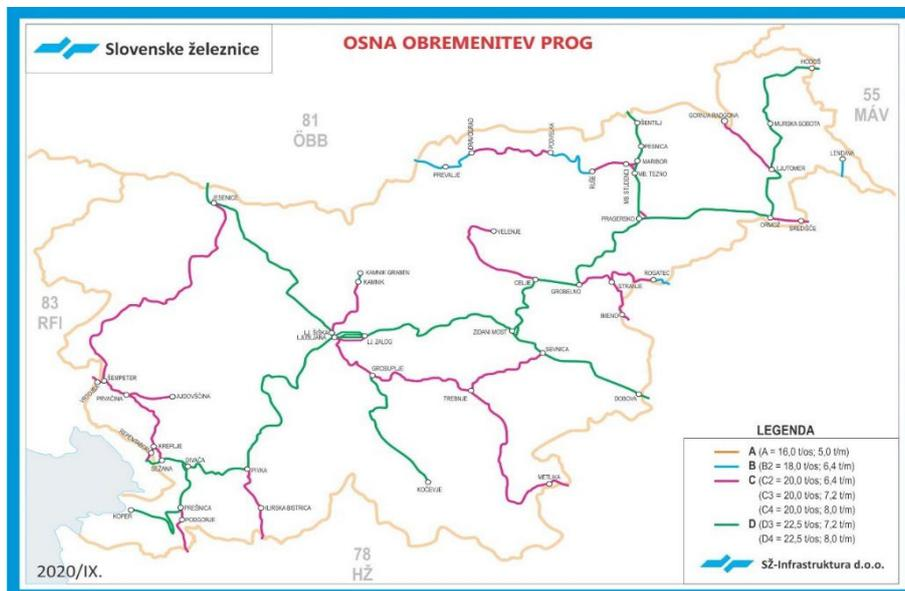
Figure 18 Line categories according to axle load [Source: gov.si teme/zelezniska-infrastruktura]
