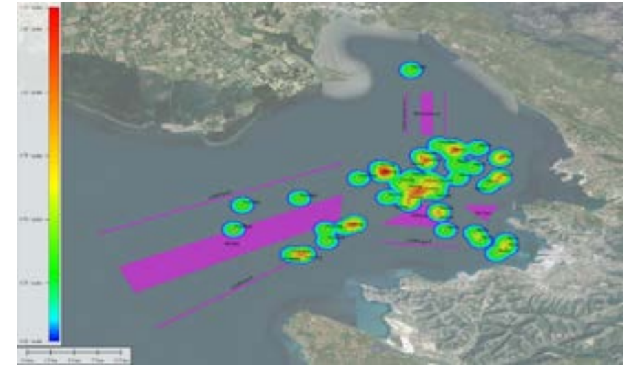
Figure 34: Simulation of possible collision locations.
